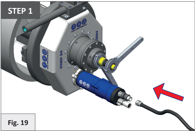
Connect the air hose to the machine pneumatic motor
